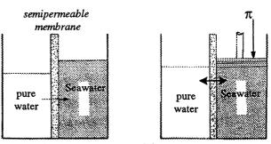
Fig. 2 osmotic pressure of the seawater system
